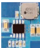
BD9D321EFJ PCB 17mm×20mm=340mm 2
