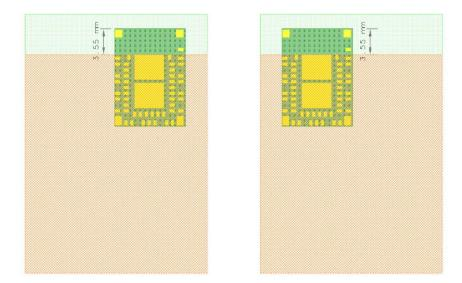
the outline of the motherboard the copper foil placeable area of the motherboard
