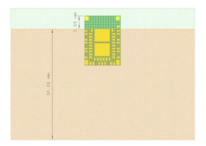
the outline of the motherboard the copper foil placeable area of the motherboard
