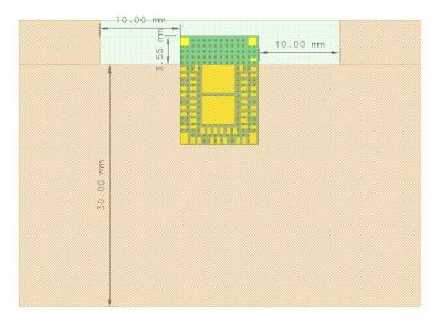
the outline of the motherboard the copper foil placeable area of the motherboard
